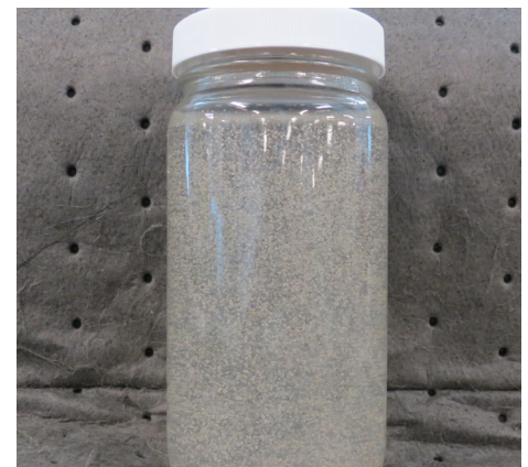
AquaLinear™ AGS service is based on a shear-thinning linear gel fluid system
